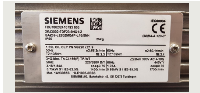
Fig. 12/9 Example, rating plate on the motor
