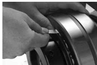
Measure RIC before installation.
